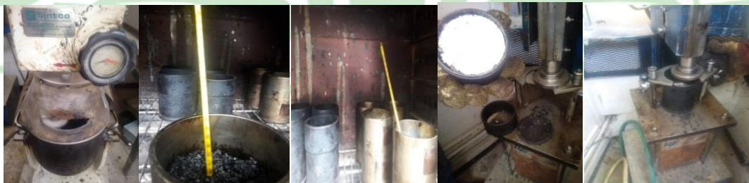
Figure 3 Preparation and compaction of samples with both additives
