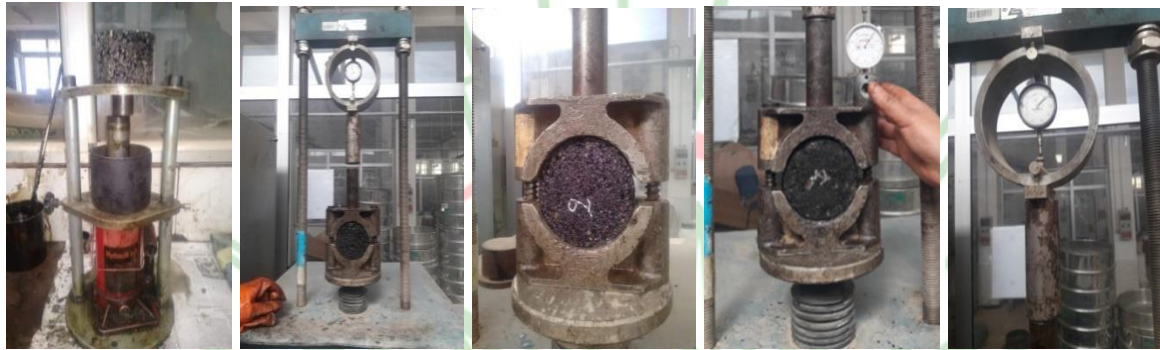
Figure 5 Crushing of the samples
