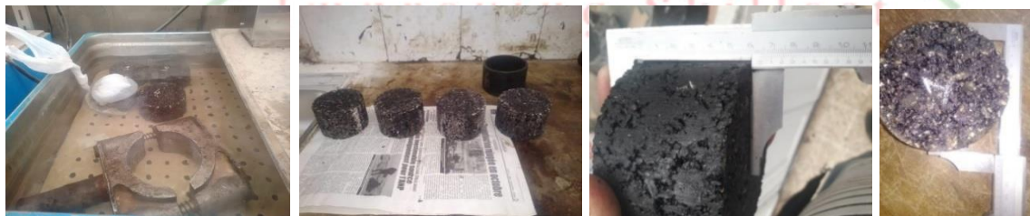
Figure 4 Preparation of modified asphalt for crushing
